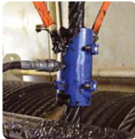
Newly installed wire rope lubricator on wire rope previously lubricated manually. Note: Even, clean penetrating distribution vs. uneven, messy coverage from previous method.
